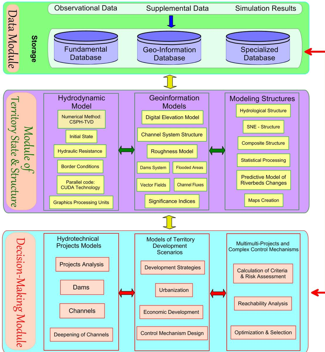
Fig. 3.2. The structure of the software package for our model of the floodplain territory control.
