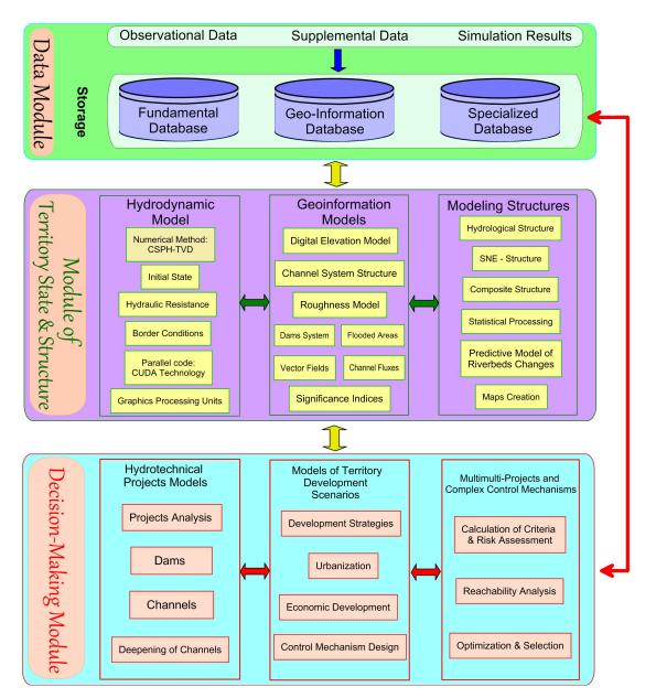
Fig. 3.2. The structure of the software package for our model of the floodplain territory control.
