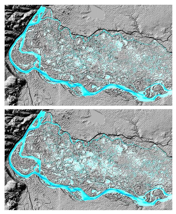
Fig. 3.5. Maps of the stably flooded area of the VAF in the period 1998-2018. Up panel: model without bypass channel with  $Q_{ch} = 0$ . Bottom panel: model with bypass channel  $Q_{ch} = 2000 \text{ m}^3 \text{ sec}^{-1}$ .
