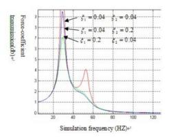
**Fig.15** Change  $\xi_2$  and  $\xi_1$  Simulation frequency—force e-coefficient of transmission
