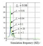
**Fig.14**  $\xi_2 = 0.06, \xi_2 = (0.01, 0.04, 0.1, 2, 20)$  Simulation frequency—force e-coefficient of transmission
