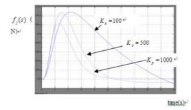
**Fig.6** Different  $K_p$  time-force curves
