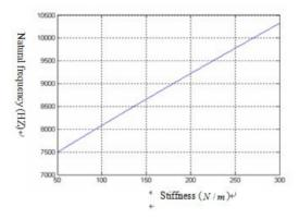
Fig.10 Curve of stiffness to natural frequency
