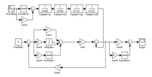
Fig.4 Block plant to simulate in Simulink of Matlab
