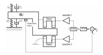
Fig.2 Theory of magnetic suspension system
