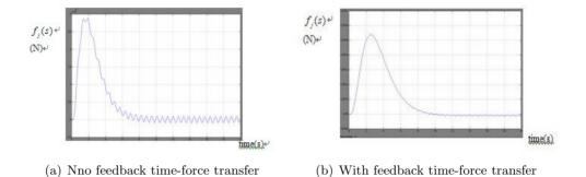
Fig.5 Comparation with before and after using magnetic suspension feed back control
