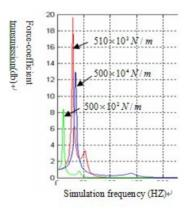
Fig.11 Influence of stiffness to force-coefficient of
