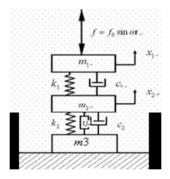
Fig.1 Model of active magnetic suspension in two-stage vibration isolation system
