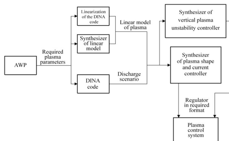
Fig. 2.1. Development of plasma control systems for ITER: AWP is an automated workplace
