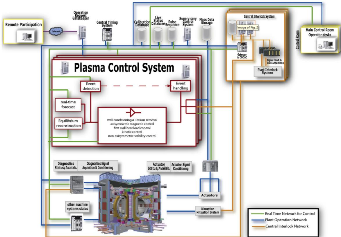
Fig. 2.3. Scheme of interfaces between plasma control systems and CODAC [21]
