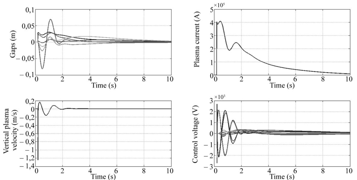
**Fig. 2.2. Real-time testbed:** (a) testbed structure; (b) real-time results of the plasma model in ITER when controlling the model by the real-time controller at minor disruption (from right to left and from top to bottom): gaps, plasma current, vertical position of the plasma, control voltages
