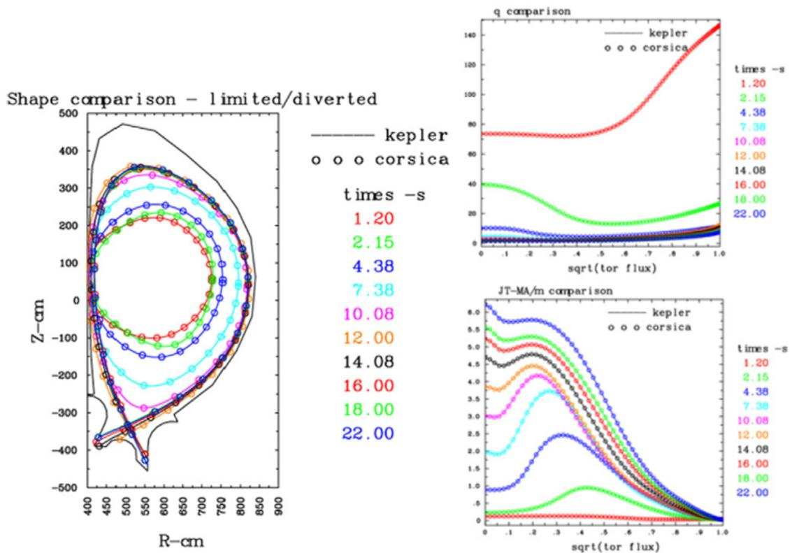
**Fig. 2.5.** Verification of the CORSICA-IMAS composition ('Kepler', solid lines) with respect to the stand-alone CORSICA code ('Corsica', circles): evolution of the plasma boundary (left), safety factor  $q$  profiles, and plasma current density (right) during plasma current rise in ITER. Both schemes provided exactly the same results: the curves completely coincided
