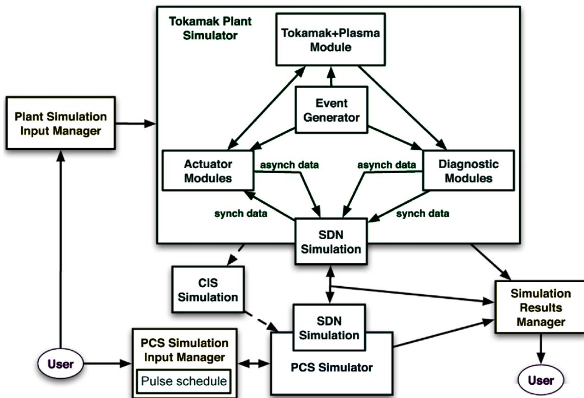
Fig. 2.4. Functional diagram of the plasma control system simulator [22, 23]
