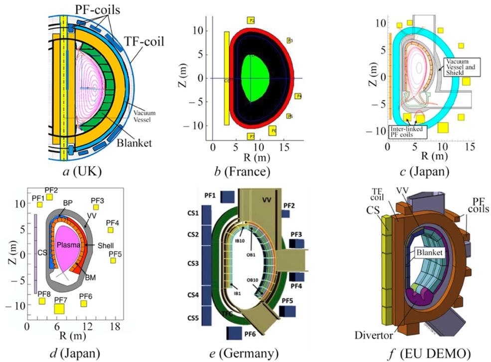
**Fig. 5.1.** Vertical cross sections of DEMO tokamaks with various poloidal system options
