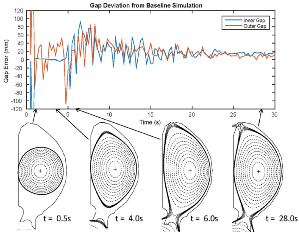
Fig. 3.1. Restoring plasma equilibrium using RT-EFIT code
