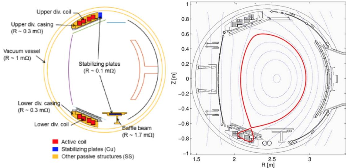
Fig. 1.2. Cross-section of the WEST tokamak: (a) design [7], (b) magnetic configuration of the plasma [8]
