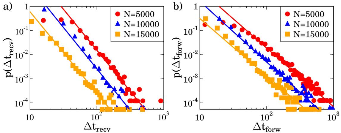
Fig. 5.3. The distribution of the average message receiving (a) and forwarding (b) time interval of vehicles. They obey a power law with exponents around 3.4 (a) and 2.5 (b) respectively, independently of the vehicle density.
