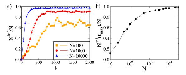
Fig. 5.1. a) Number of informed agents (vehicles) as a function of time for different numbers of agents. After a short time period a saturation is achieved at a quite high value. b) The previous saturation level depends on the number of vehicles in the system (of course more smart vehicle leads to higher level of awareness).
