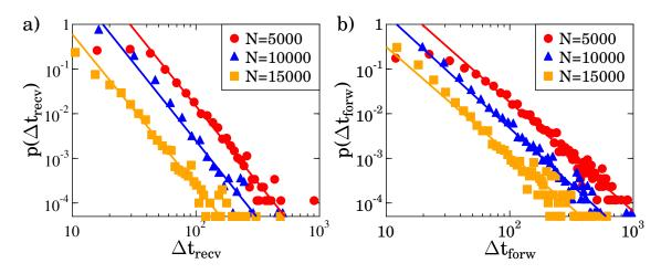
Fig. 5.3. The distribution of the average message receiving (a) and forwarding (b) time interval of vehicles. They obey a power law with exponents around 3.4 (a) and 2.5 (b) respectively, independently of the vehicle density.
