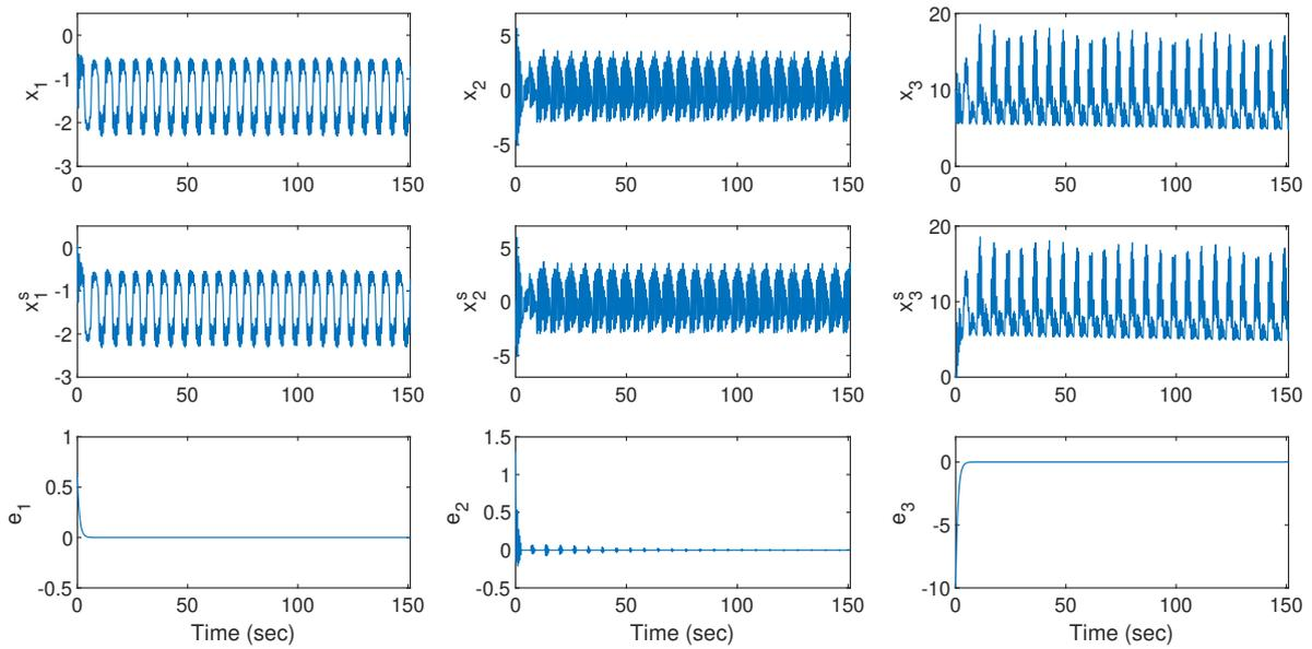
Fig. 4.3. Proposed method (Gyro-Gyro): row 1: Master system states, row 2: Slave gyro system states, row 3: Synchronization error
