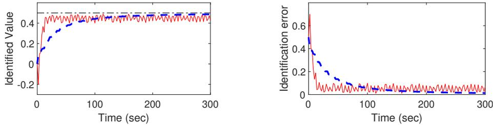
Fig. 4.5. Gyro-gyro synchronization: Left: Parameter identification, Right: Identification error; Dashed-dotted line (black): Nominal value, Dashed line (blue): Proposed method, Solid line (red): Method of [30]
