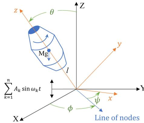
Fig. 2.1. Schematic of a gyroscope on a vibrating base
