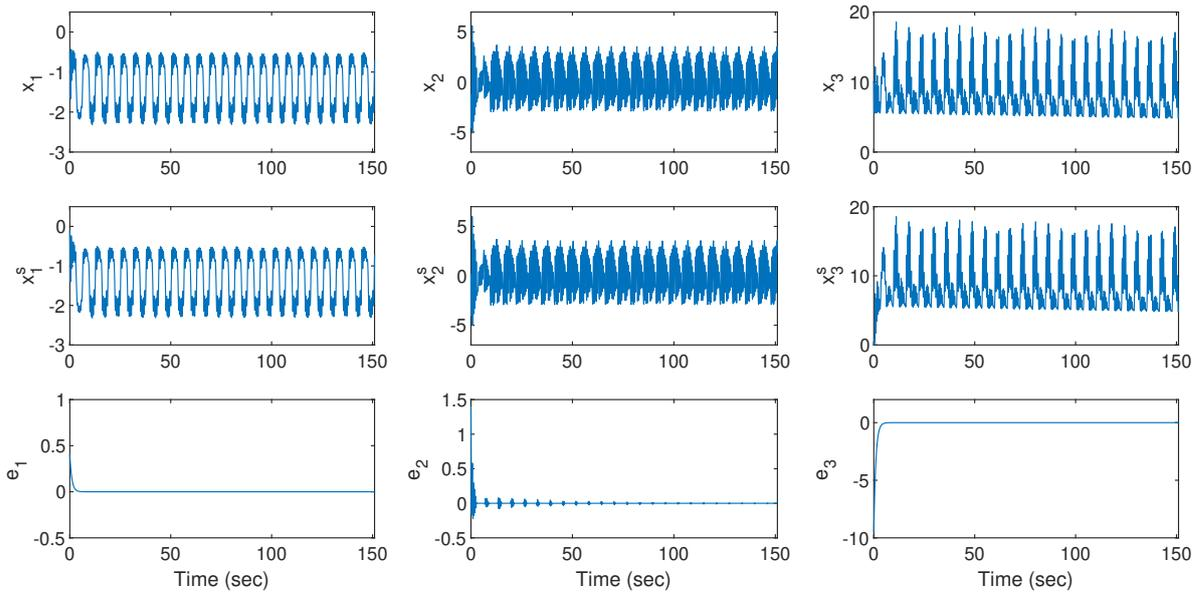
Fig. 4.4. Proposed method (Gyro-Rössler): row 1: Master system states, row 2: Slave gyro system states, row 3: Synchronization error
