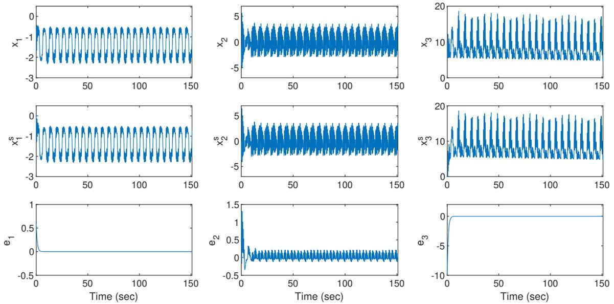
Fig. 4.2. Method of [30]: row 1: Master system states, row 2: Slave gyro system states, row 3: Synchronization error
