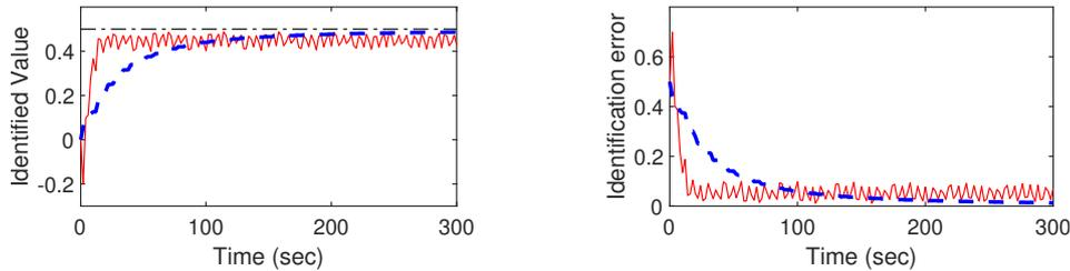
Fig. 4.6. Gyro-Rössler synchronization: Left: Parameter identification, Right: Identification error; Dashed-dotted line (black): Nominal value, Dashed line (blue): Proposed method, Solid line (red): Method of [30]
