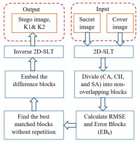
Fig. 1. SLT-EM1 data embedding procedure
