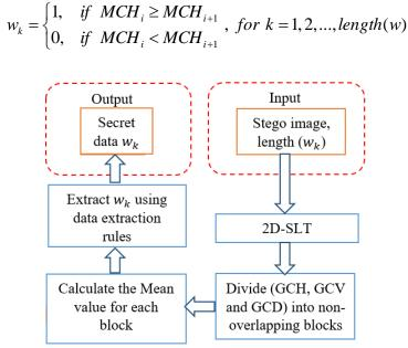
Fig. 4. SLT-EM2 data extraction procedure
