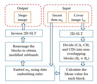
Fig. 3. SLT-EM2 data embedding procedure
