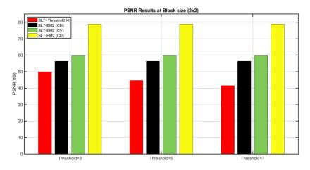
Fig. 10. Visual quality comparison of SLT-EM2 with threshold method at block size (2×2).
