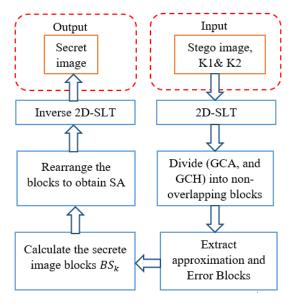
Fig. 2. SLT-EM1 data extraction procedure
