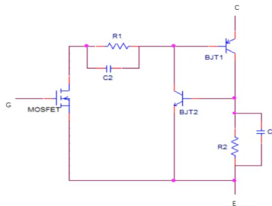
**Fig. 5.4.** Improved IGBT Model equivalent circuit.
