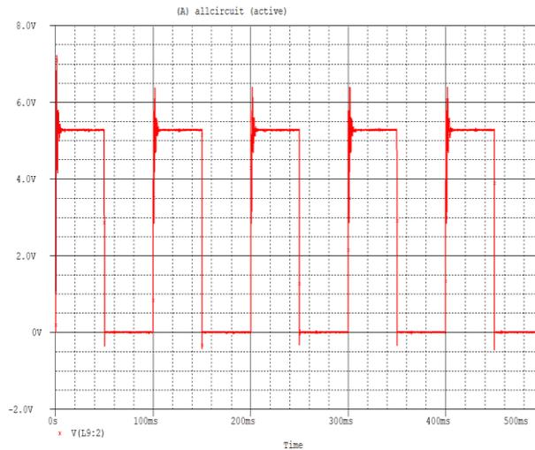
**Fig. 6.2.** Simulation of modified circuit based on existing LVDC SSCB model overvoltage without snubber circuit.
