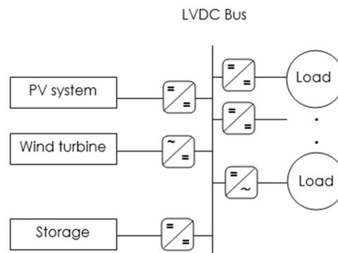
**Fig. 2.1.** Conceptualization of the LVDC bus microgrid system.
