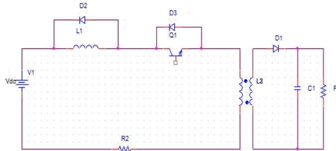
Fig. 4.1. Proposed LVDC circuit breaker mode.
