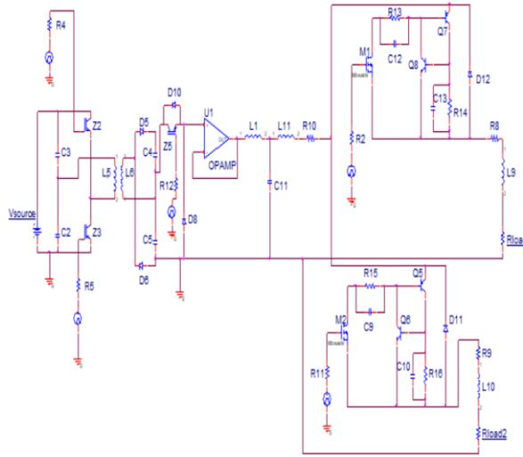
**Fig. 6.1.** Modified circuit schematic based on existing LVDC SSCB without snubber circuit.
