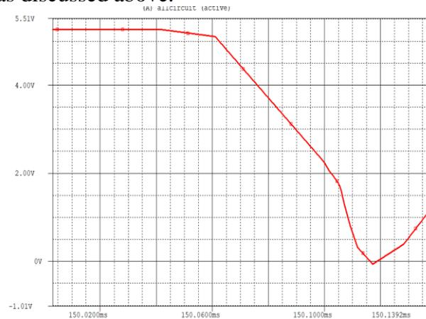
**Fig. 6.5.** Proposed SSCB model switching time.
