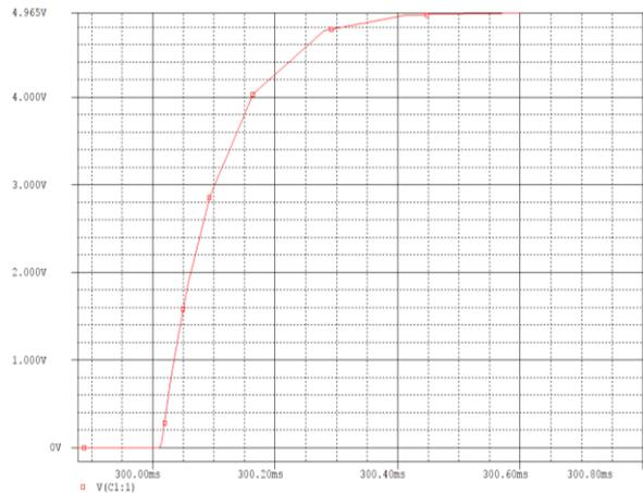
**Fig. 5.6.** Switching time of the improved IGBT Model.
