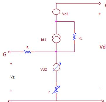
Fig. 4.2. LVDC model of IGBT.
