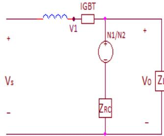
**Fig. 4.3.** Proposed LVDC circuit breaker mode.
