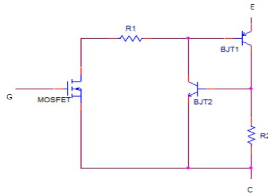
Fig. 5.1. P IGBT Model equivalent circuit.
