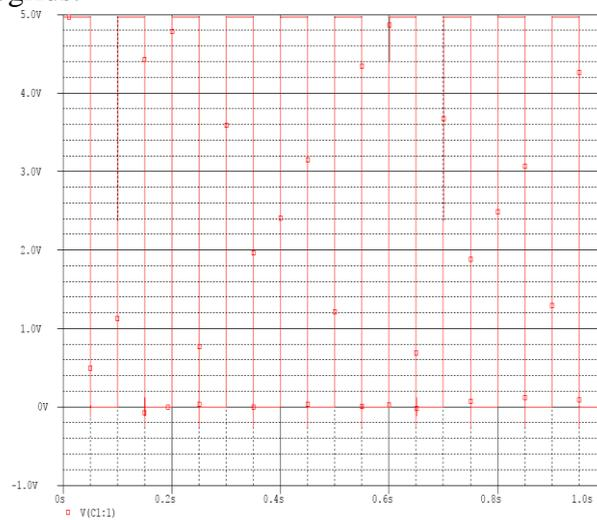
**Fig. 5.5.** Switching time of IGBT model.
