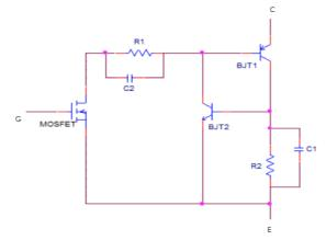
Fig. 5.4. Improved IGBT Model equivalent circuit.
