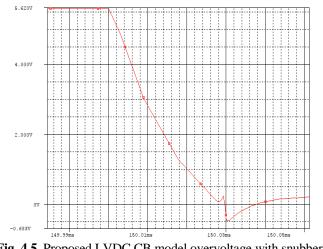
Fig. 4.5. Proposed LVDC CB model overvoltage with snubber.
