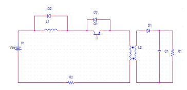
Fig. 4.1. Proposed LVDC circuit breaker mode.
