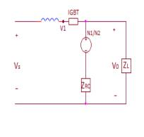
Fig. 4.3. Proposed LVDC circuit breaker mode.
