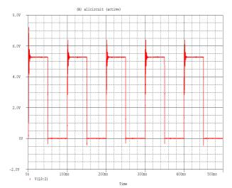
Fig. 6.2. Simulation of modified circuit based on existing LVDC SSCB model overvoltage without snubber circuit.
