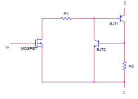
Fig. 5.1. P IGBT Model equivalent circuit.
