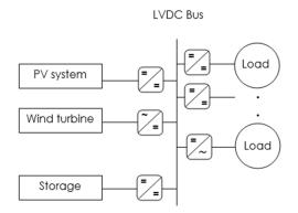
Fig. 2.1. Conceptualization of the LVDC bus microgrid system.
