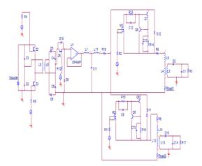
Fig. 6.3. Circuit schematic of proposed LVDC SSCB with snubber circuit.
