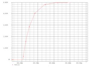
Fig. 5.6. Switching time of the improved IGBT Model.
