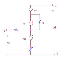
Fig. 4.2. LVDC model of IGBT.
