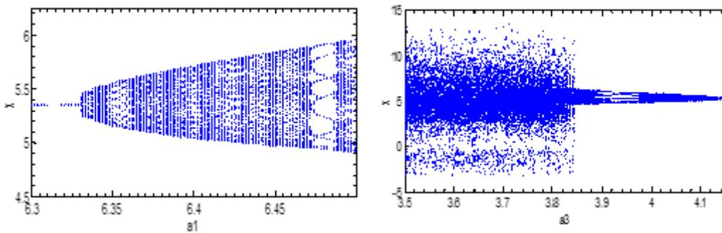
Fig. 2.2. Bifurcation diagrams of control parameters  $\alpha_1, \alpha_3$
