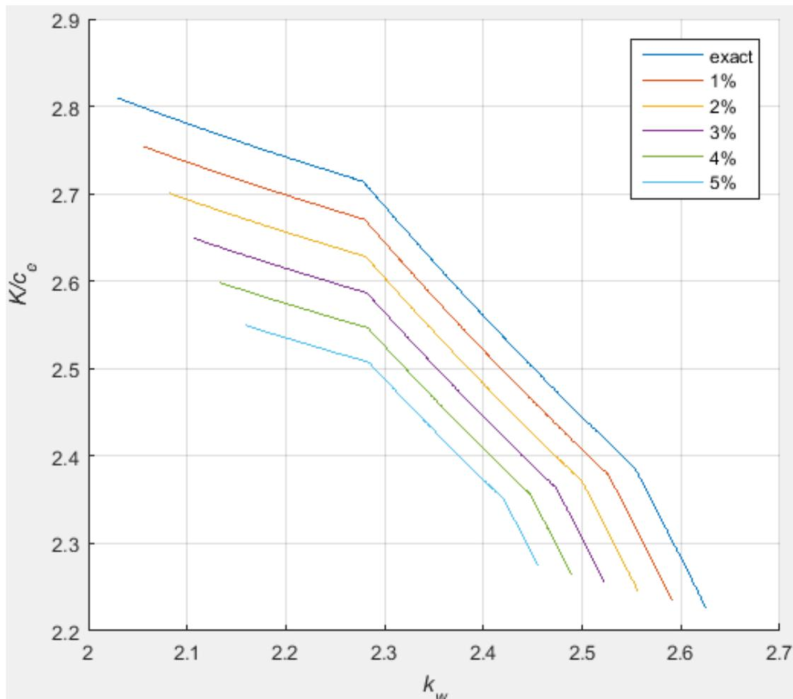
Fig. 5.3. Approximation of Pareto fronts obtained by the Monte Carlo method
