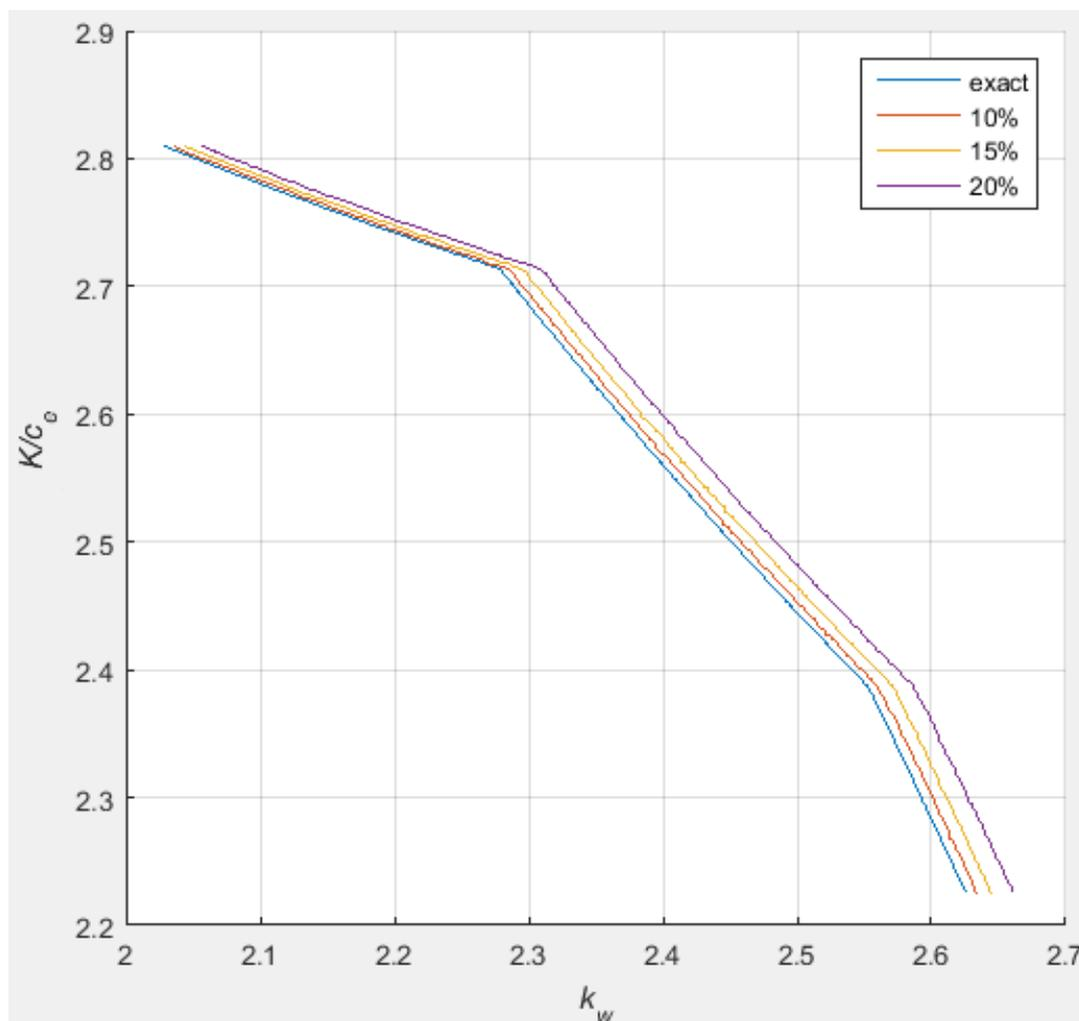
Fig. 5.1. Approximation of the Pareto fronts for different ranges of uncertain input parameters
