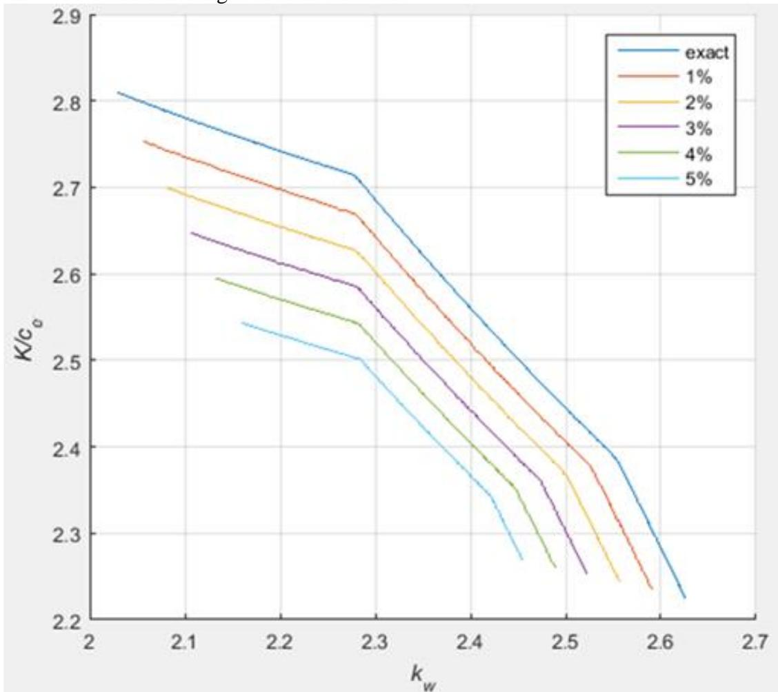
Fig. 5.2. Approximation of the Pareto fronts for different ranges of uncertain design parameters
