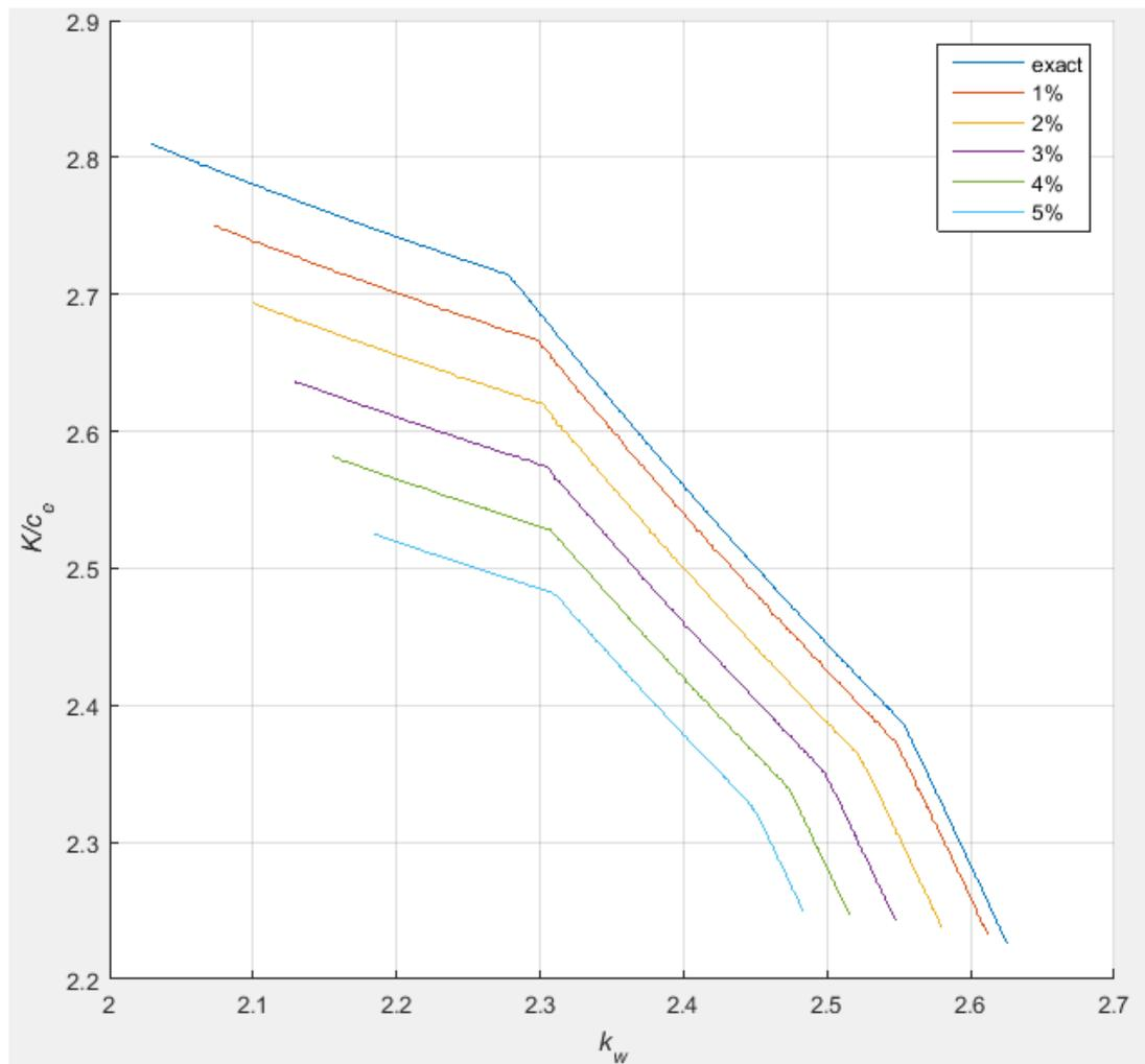
Fig. 5.4. Approximation of Pareto fronts for various ranges of uncertain design parameters with a range of uncertain input parameters 15%.
