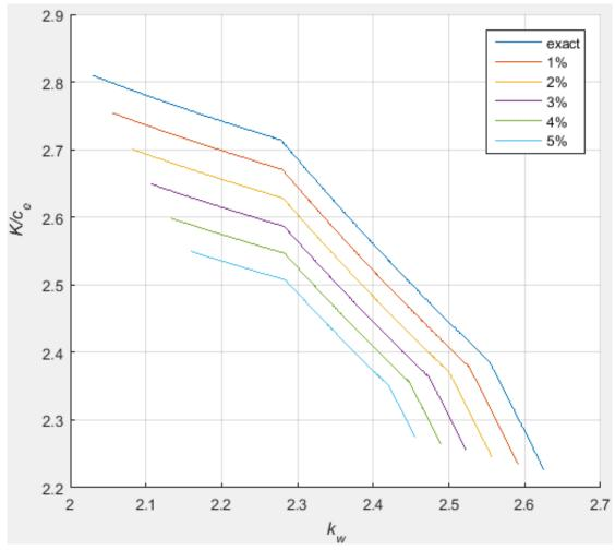
Fig. 5.3. Approximation of Pareto fronts obtained by the Monte Carlo method
