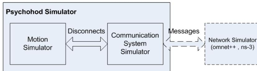
Fig. 4.1. Conjugation of the agents' motion simulator, the communication simulator, and (optional) a network simulator
