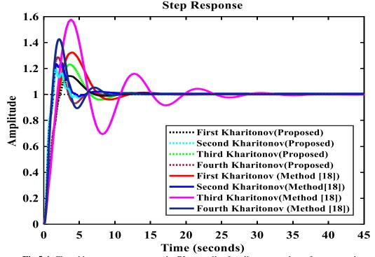
**Fig.5.4.** Closed loop step response to the PI controller for all extreme plants for proposed method and the method given in[18].
