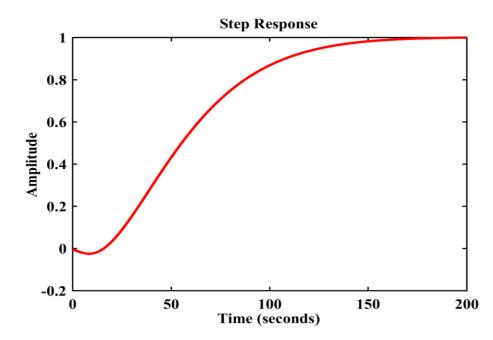
Fig.5.15. Closed loop step response to the PID controller for changes in the uncertain parameter to determine the robustness with time delay for the proposed method
