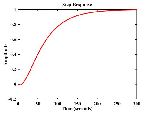
Fig.5.13. Closed loop step response to the PI controller for changes in the uncertain parameter to determine the robustness for proposed method
