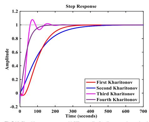
Fig.5.14. Closed loop step response with PID controller for all extreme plants using the proposed method with time delay.
