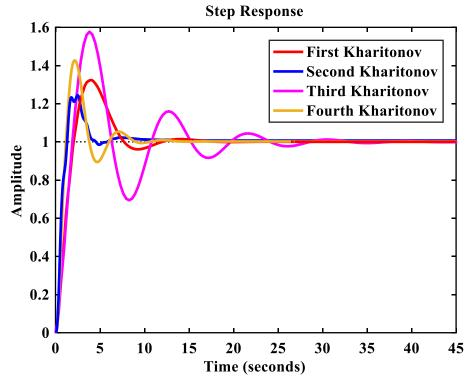
Fig.5.3. Closed loop step response to the PI controller for all extreme plants using the method given in [18].
