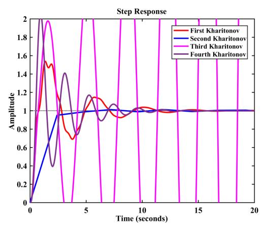
Fig.5.1. Closed loop step response with PI controller for all extreme Plants using the Ziegler-Nichols
