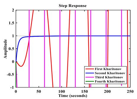
Fig. 5.9. : Closed loop step response to the PI controller for all extreme plants using Ziegler-Nichlos method with time delay.
