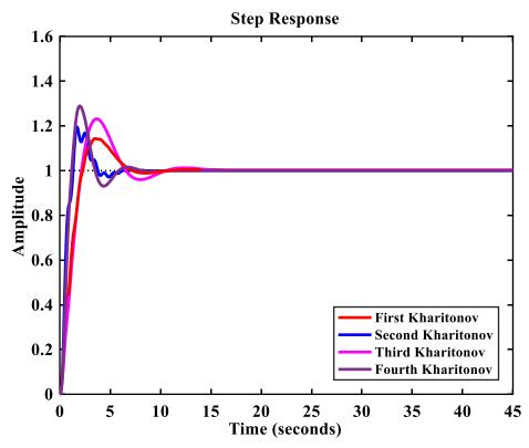
Fig. 5.2. Closed loop step response to the PI controller for all extreme plants using the proposed method.
