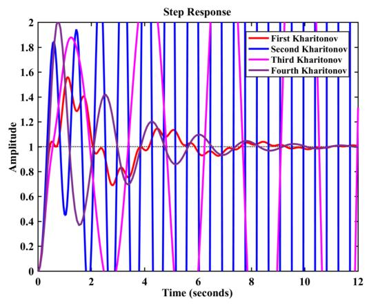
Fig.5.6. Closed loop step response with PID controller for all extreme Plants using the Ziegler-Nichols
