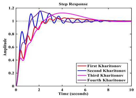
Fig.5.7. Closed loop step response with PID controller for all extreme Plants using the proposed method.
