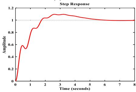
Fig.5.8. Closed loop step response to the PID controller for changes in the uncertain parameter to determine the robustness of the proposed method
