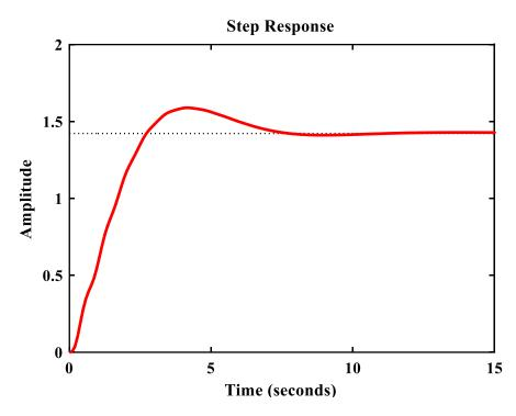
**Fig.5.5.** Closed loop step response to the PI controller for changes in the uncertain parameter to determine the robustness for proposed method
