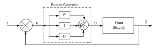
Fig.3.1. Block diagram of interval Plant with a Robust Controller
