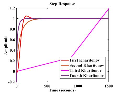
Fig.5.12. Closed loop step response to the PI controller for all extreme plants using the existing method [30].
