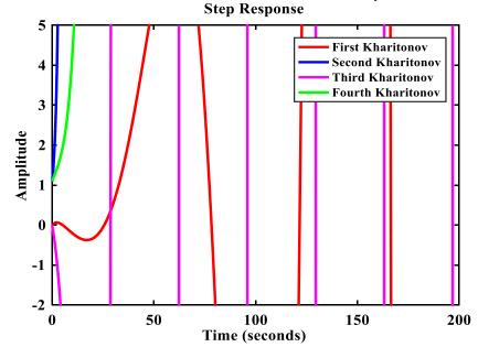
Fig. 5.10: Closed loop step response to the PID controller for all extreme plants using Ziegler-Nichlos method with time delay.
