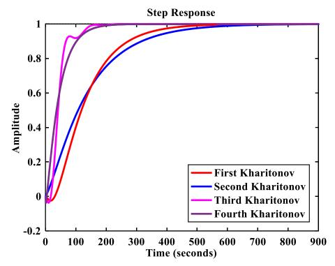
Fig.5.11.Closed loop step response with a PI controller for all extreme plants using proposed method with time delay.
