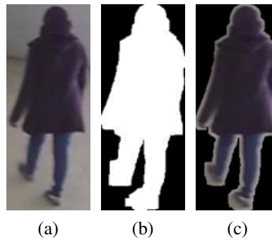
Fig. 4.8. The multiplication of detected object with its mask, (a) Detected object, (b) Mask of detected object and (c) Results of multiplication
