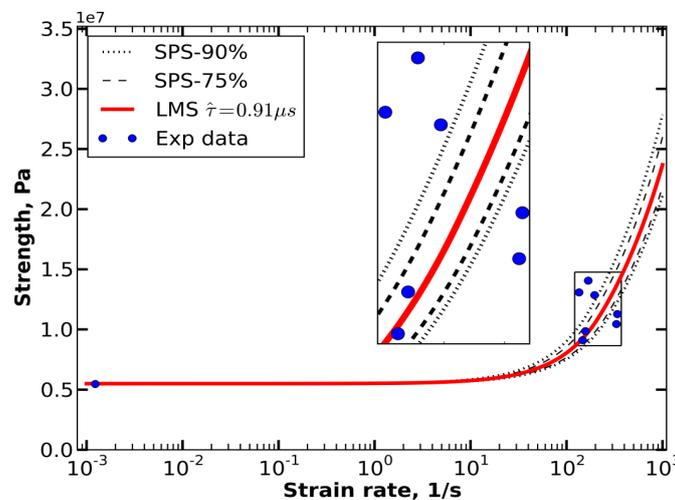
Fig. 3. Dynamic fracture of Coelga marble [18]. Red line is plotted by LMS method; dotted lines are plotted by SPS procedure for  $\tau_{0.9} \in [0.39; 0.89] \mu s$ ; Dashed lines -  $\tau_{0.75} \in [0.48; 0.78] \mu s$
