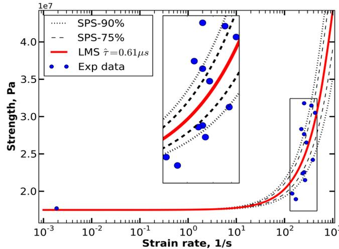
Fig. 2. Dynamic fracture of gabbro-diabase [18]. Red line is plotted by LMS method; dotted lines are plotted by SPS procedure for  $\tau_{0.9} \in [0.39; 0.89] \mu s$ ; Dashed lines -  $\tau_{0.75} \in [0.48; 0.78] \mu s$
