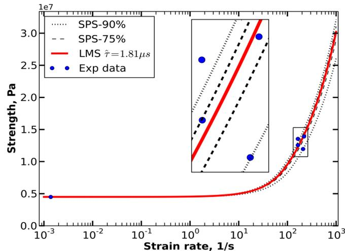
Fig. 4. Dynamic fracture of Pervouralsky marble [18]. Red line is plotted by LMS method; dotted lines are plotted by SPS procedure for  $\tau_{0.9} \in [0.39; 0.89] \mu s$ ; Dashed lines -  $\tau_{0.75} \in [0.48; 0.78] \mu s$
