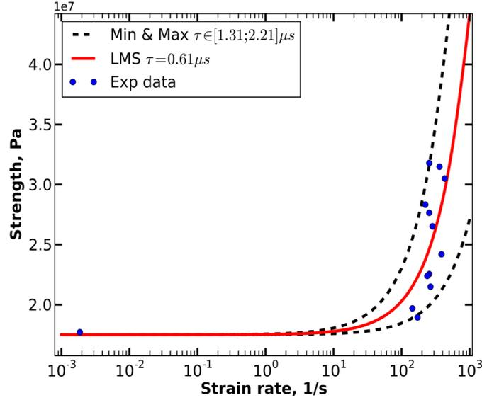
Fig. 1. Dynamic fracture of gabbro-diabase [18]. Blue points are experimental data. Lines are theoretical curves plotted by the incubation time fracture criterion: solid line - least mean squares method; dashed lines - min & max robust method
