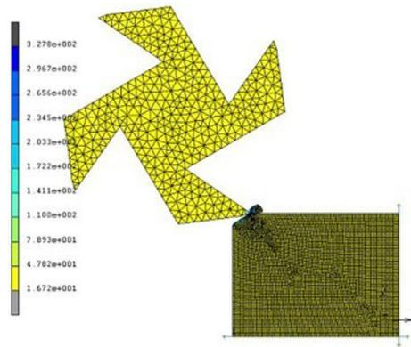
**Fig.7** The simulation of up-milling
