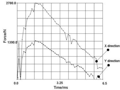
**Fig.8** The milling force of down milling
