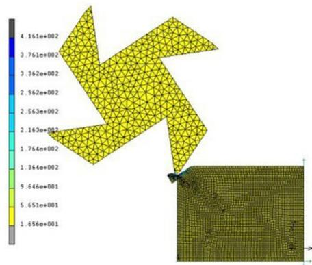
Fig.6 The simulation of down milling
