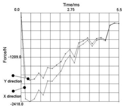
**Fig.9** The milling force of up-milling
