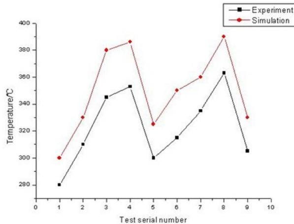
**Fig.11** The comparison of cutting temperature
