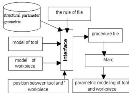
**Fig.3** The block diagram of modeling process
