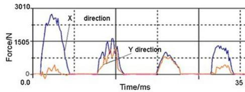
**Fig.10** The simulation of cutting force of down milling
