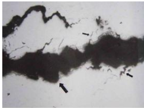
Fig.3 Metallographic grinding in the surface morphology of the cracks
