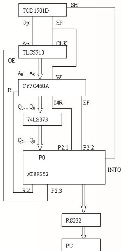
**Fig.3** Block diagram of hardware system
