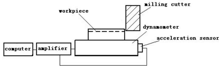
**Fig.2** Diagram of force measuring principle
