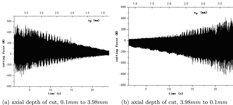
Fig 5 Radial cutting force of varying cutting-depth test
