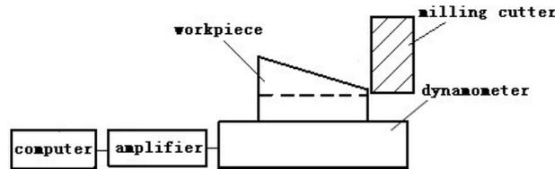
Fig.4 Diagram of varying axial depth of cut test principle
