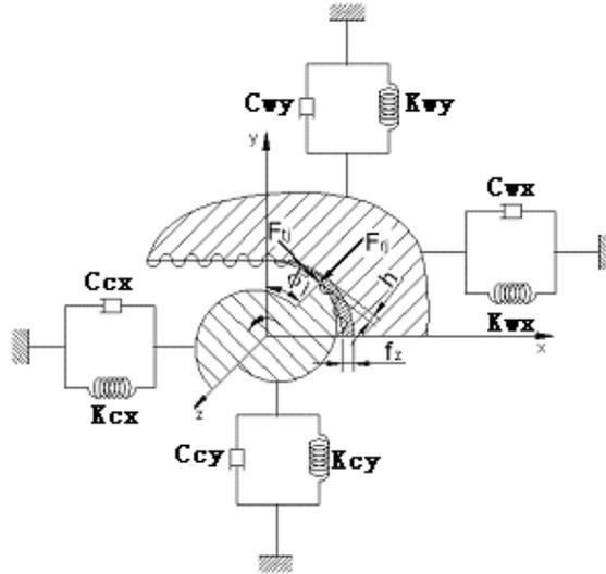
**Fig.1** Dynamic milling model of thin-walled workpieces
