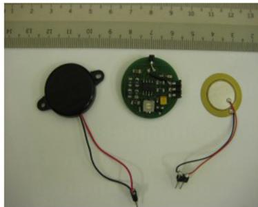
Conditioning circuit for Piezo sensors
