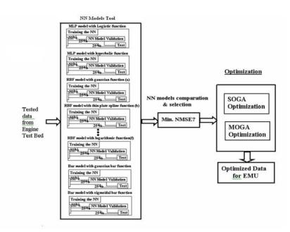
Fig.6 The structure of the optimisation system of the engine performance
