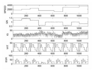
**Fig.10** Input data set: SPEED (rpm), GN(%), IG(degree), VVT(degree) and EGR(%)
