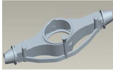
Fig.4. The new pouring system and 3D solid model
