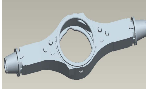
Fig.1. Structure of the rear axle casing
