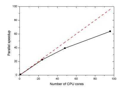
Fig. 3. The dependence of the parallel speedup of the test model on the number of CPU cores.
