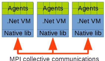
**Fig. 1.** The agents of the model are implemented using C# programming language and run in .Net virtual machine. The interaction between VM instances is implemented through the native library and MPI library.
