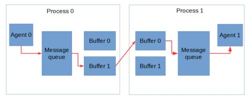
**Fig. 2.** The message sending procedure. The message from Agent 0 is transmitted first to Message queue of process 0, then the message is serialized to outgoing buffer for sending to process 1, then the buffers are exchanged between processes and the outgoing buffer number 1 becomes the incoming buffer number 0 on MPI process number 1, then the message is deserialized and delivered to Agent 1 by the message queue.
