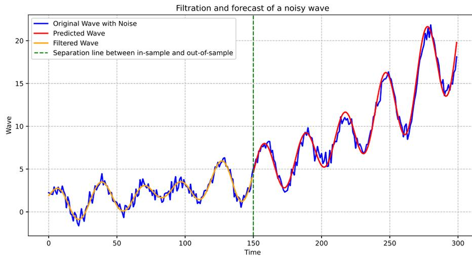
Fig. 3.3. Filtration and forecast of a noisy wave with exponential trend.
