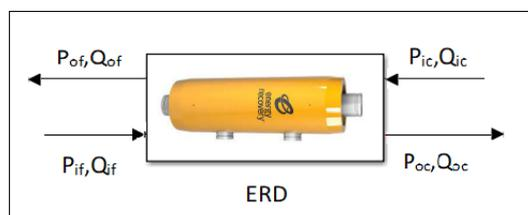
Fig. 5.1. The ERD system's inputs and outputs
