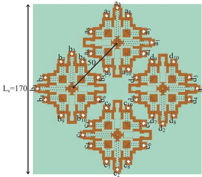
Fig. 5. 2X2 Dual Polarized reconfigurable S-Band array (4X4 C-Band array)
