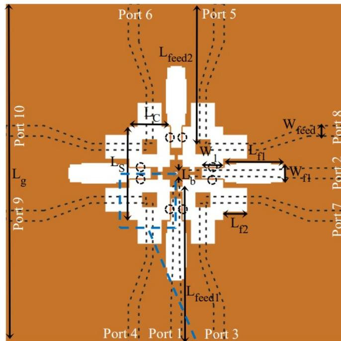
Fig. 4. Configuration of reconfigurable dual-polarized wideband slot ring antenna/array
