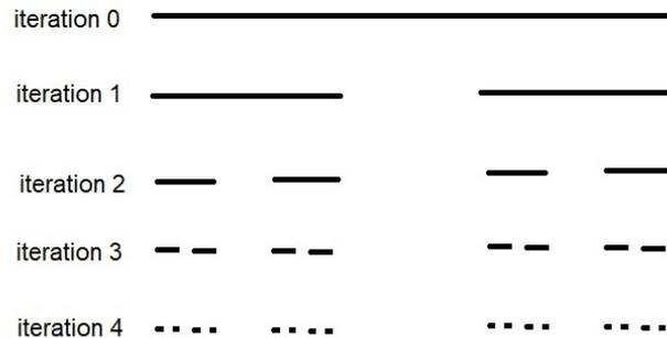
Fig. 2. The first four iterations in the construction of the Cantor set array.
