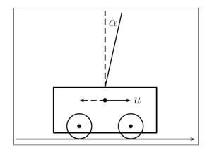
Fig. 6.9. Inverted pendulum on the cart
