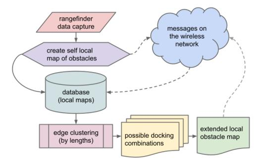
Fig. 3.2. Algorithm cycle to obtaining an extended local obstacle map.
