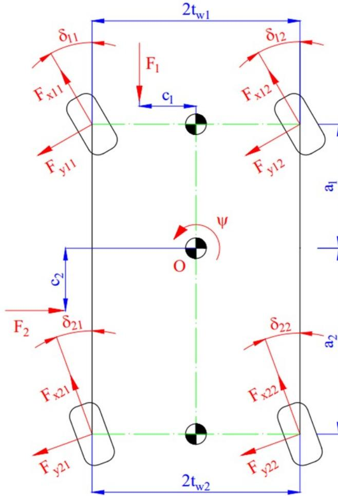
Fig. 2. Model of the nonlinear double-track dynamics.
