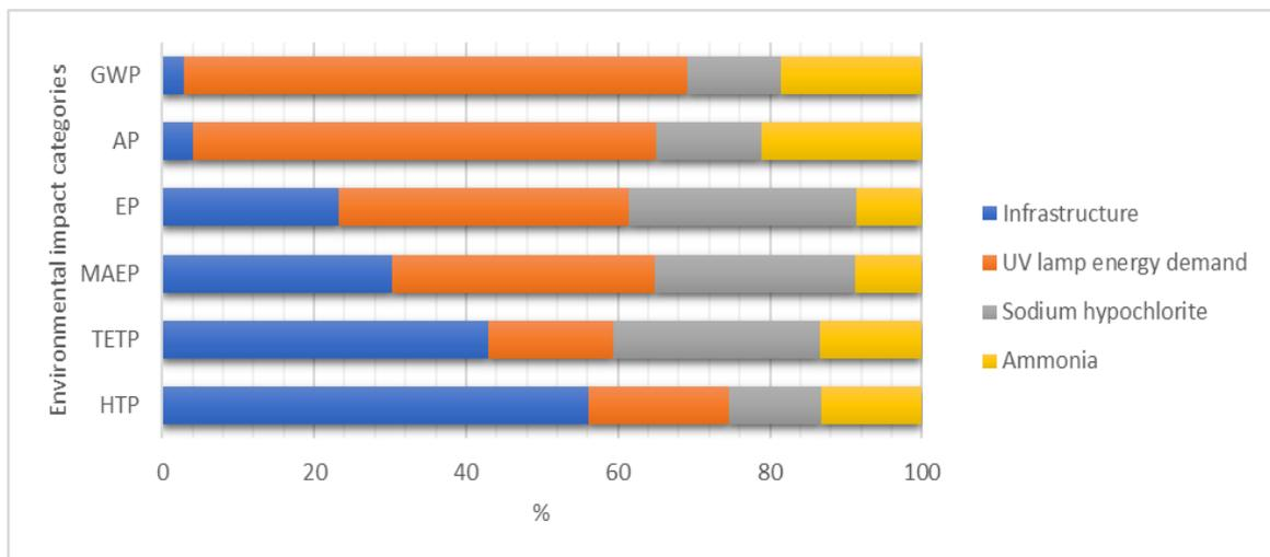
**Figure 5.** The contribution of infrastructure, energy consumption of UV lamps and chemicals to environmental impact of the UV disinfection system at a dose of 30 mJ/cm<sup>2</sup>
