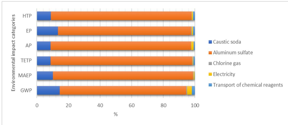
**Fig. 2.** Contribution of caustic soda, aluminum sulfate, chlorine gas, electricity, and transport of chemical reagents to the environmental impact at the Latacunga water treatment plant.
