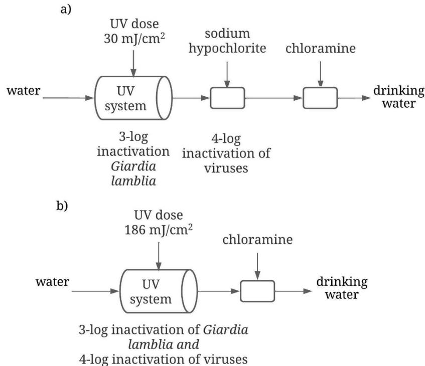
Fig. 4. Schemes of the proposed disinfection processes based on UV-radiation.
