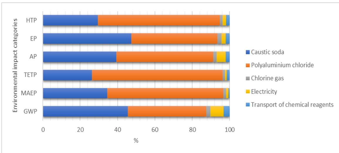
**Figure 3.** Contribution of caustic soda, polyaluminium chloride, chlorine gas, electricity, and transport of chemical reagents to the environmental impact at the Pedro Vicente Maldonado water treatment plant.
