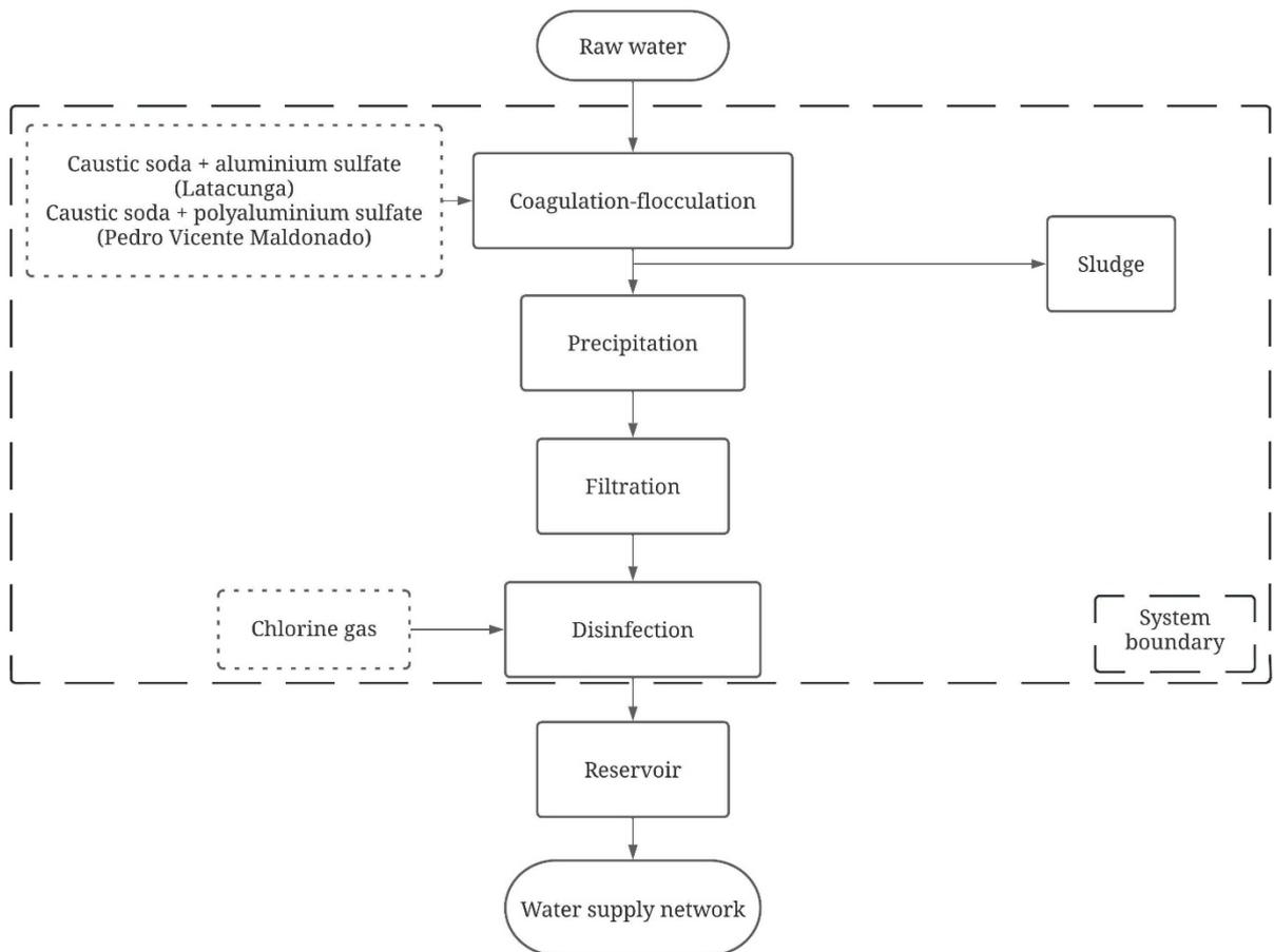
**Fig. 1.** System boundaries of the process at the studied water treatment plants. The chemical reagents used for each process are indicated by a dotted line
