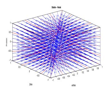
Fig. 3.3. Three-dimensional vector plot of the system of linear differential equations where arrows showing the direction (blue colour) and streamlines (red colour) converging to the equilibrium point (0, 0, 0) which displays the stability of the system as a stable-node. The eigenvalues of the system are (-0.7655, -0.1016, -0.8603).
