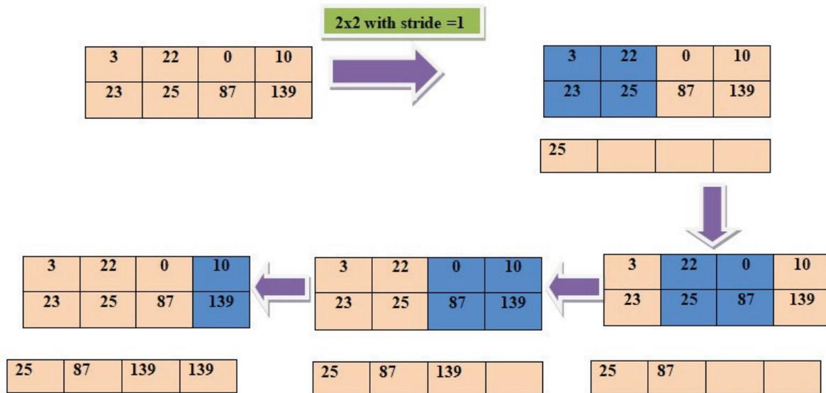
Fig. 2.5. Operation of Max pooling
