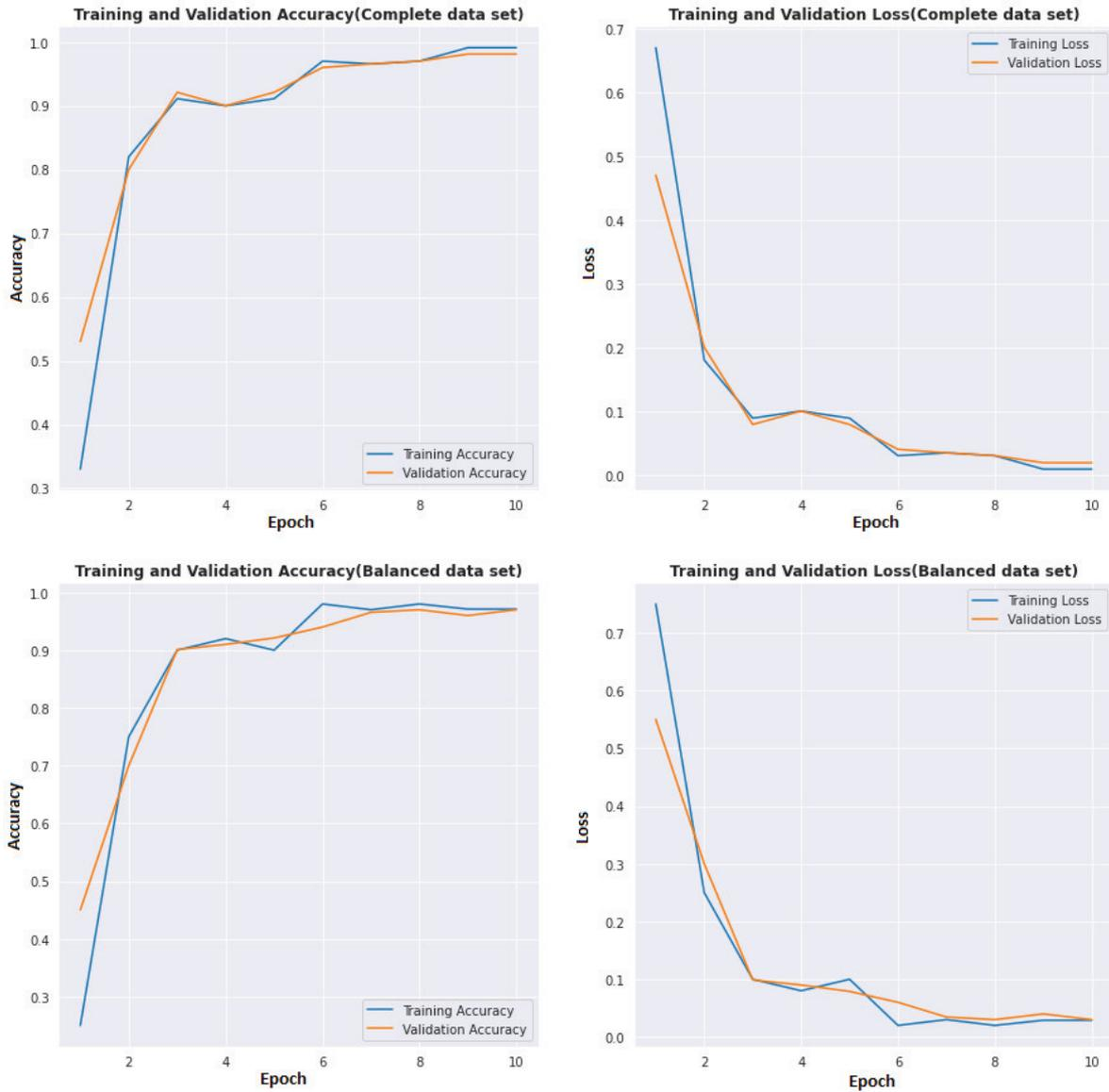
Fig. 3.7. Training and Validation Accuracy and Loss plot for complete data set and balanced data set
