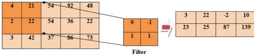
Fig. 2.4. 2D convolution operation
