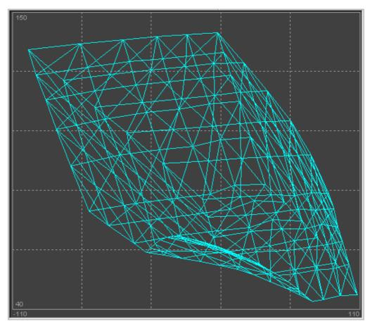
Fig. 1. A piecewise linear approximation of the gamut boundary for a three-dimensional printing device
