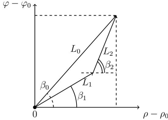
Fig. 5.3. The mobile vehicle in the  $(\rho, \varphi)$  coordinate system.
