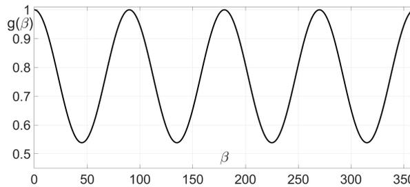
Fig. 6.5. Radiation pattern of the mobile vehicle as a function of  $\beta$
