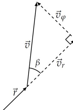
Fig. 3.2. Rectangular triangle of velocity vectors  $\vec{v}$ ,  $\vec{v}_r$  and  $\vec{v}_\varphi$ .
