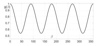
Fig. 6.5. Radiation pattern of the mobile vehicle as a function of  $\beta$
