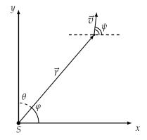
Fig. 3.1. The moving object in the Cartesian coordinate system with sensor S.
