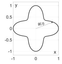
Fig. 6.4. Radiation pattern of the mobile vehicle on Cartesian plane
