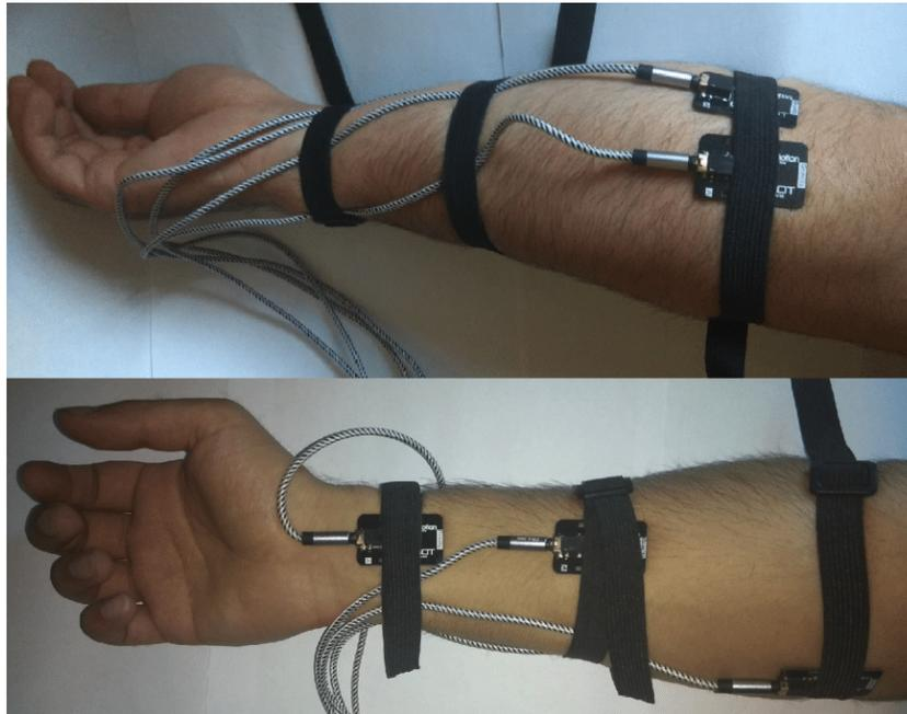
Fig. 2.1. Location of EMG sensors.
