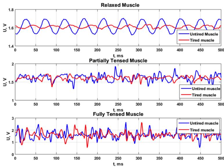
Fig. 3.5. Comparison of EMG shapes of untired and tired muscles.
