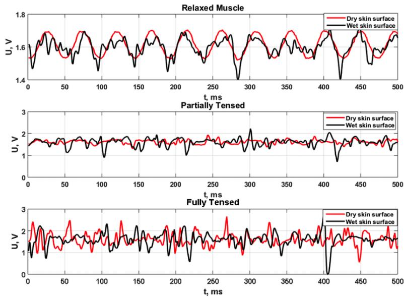
Fig. 3.7. Comparison of waveforms with perspiration.
