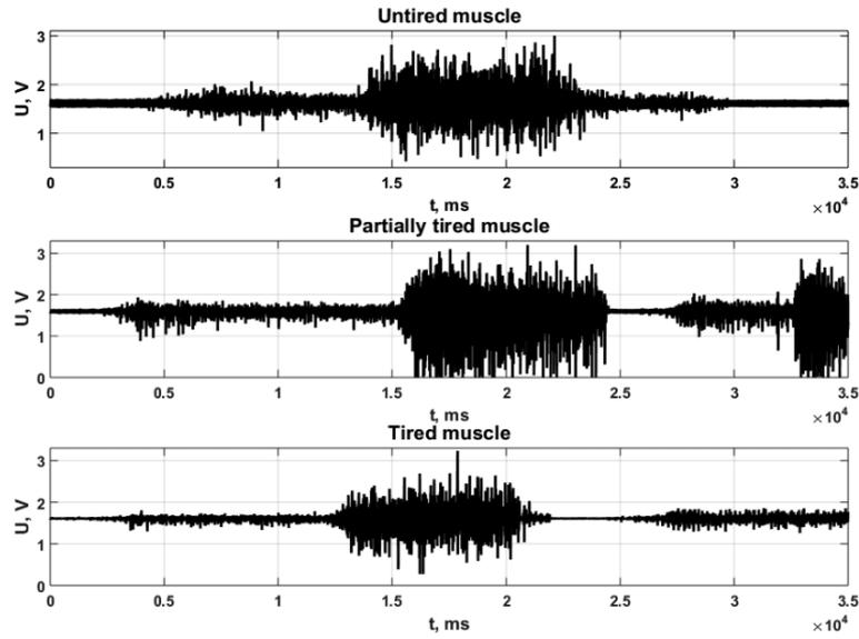
Fig. 3.4. Comparison of muscle fatigue charts: a.) untired muscle; b.) partially tired muscle; c.) tired muscle.
