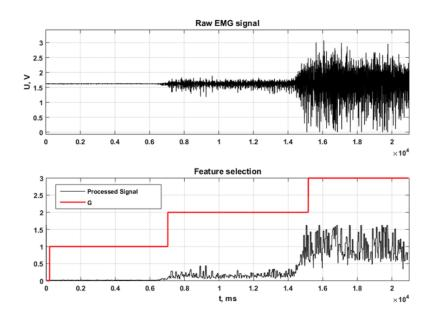
Fig. 2.2. EMG data processing: a.) Raw signal. b.) Results of muscle activity recognition using window method.
