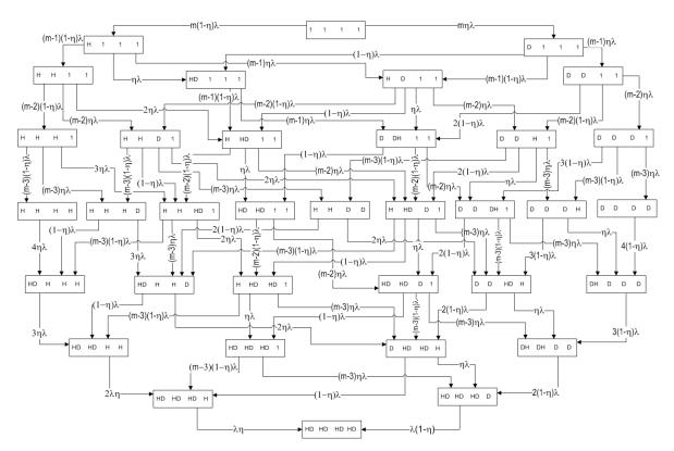
Fig. 3.5. Graph representation of the MRM over target operation phase  $(1 \le m \le 4, 1 \le k \le m)$ .
