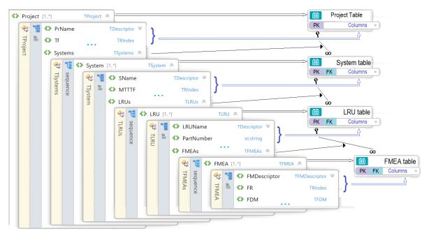
Fig. 2.1. TXSD to database schema conversion (FK - foreign key, PK - primary key).
