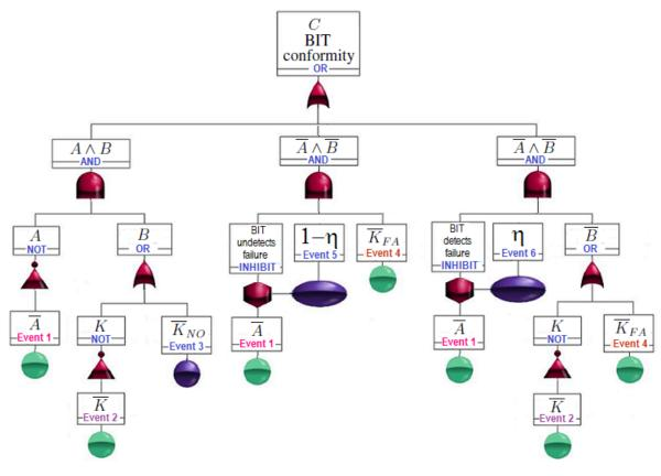
Fig. 3.3. Fault tree model of BIT conformity.
