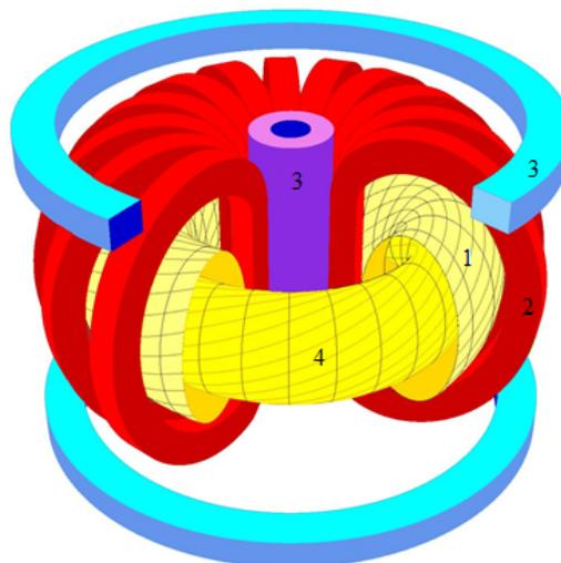
**Fig. 1.** Vertically elongated tokamak without an iron core: 1 is the vacuum vessel; 2 is the toroidal field coil; 3 is the poloidal field inner and outer coils; 4 is plasma and helical magnetic lines (© ITER Project Center, Russia)
