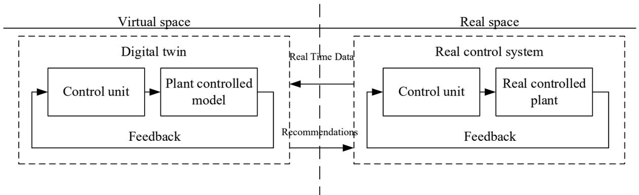
**Fig. 5.** Digital twin of feedback control system of real dynamical plant [IFAC 2020 WC]
