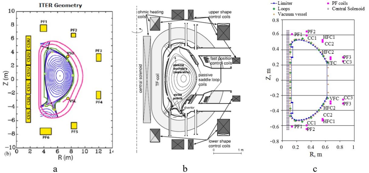
Fig. 3. Vertical cross-sections of (a) ITER [22], (b) ASDEX Upgrade [23], (c) Globus-M2 [24]
