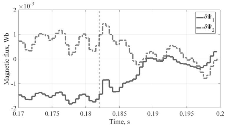
Fig. 9. Deviations of the flux in the desired location of the plasma separatrix (Fig. 4) for the shot № 31648 in discrete time [15]
