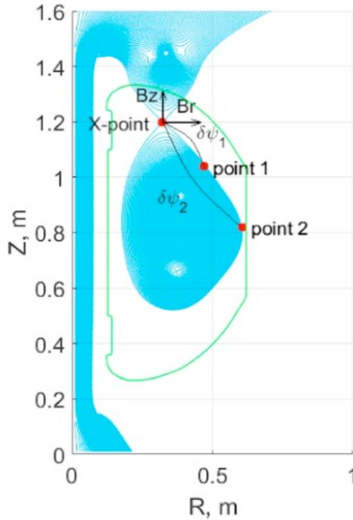
Fig. 7. The idea of the isoflux plasma shape control [15]
