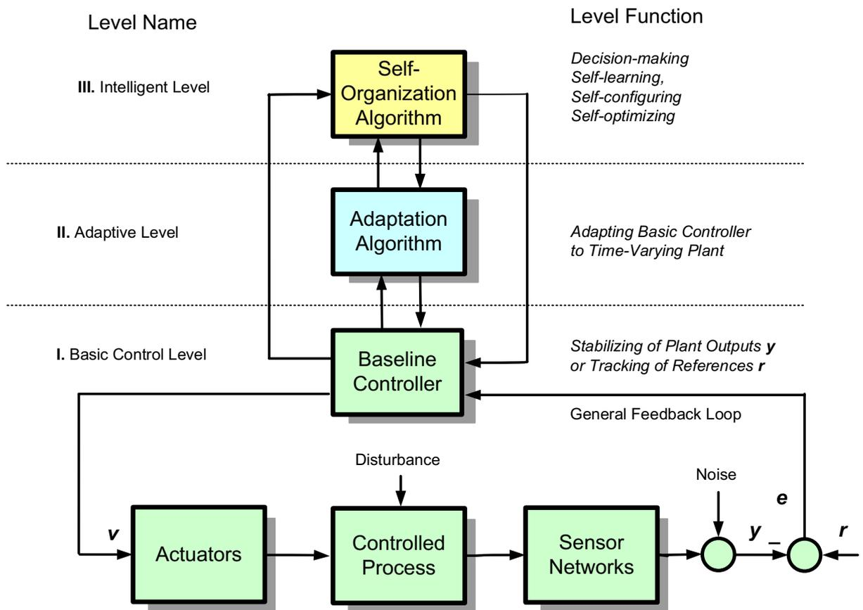
Fig. 2. General configuration of three levels hierarchical control system [8]
