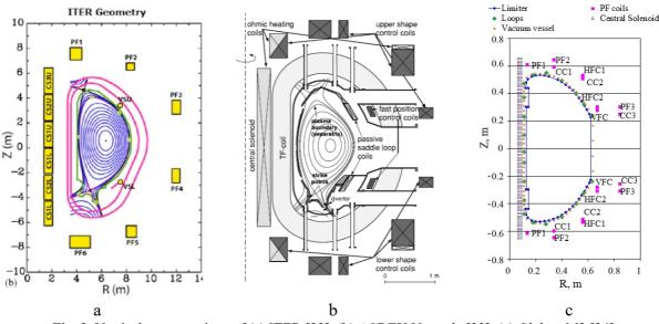
Fig. 3. Vertical cross-sections of (a) ITER [22], (b) ASDEX Upgrade [23], (c) Globus-M2 [24]
