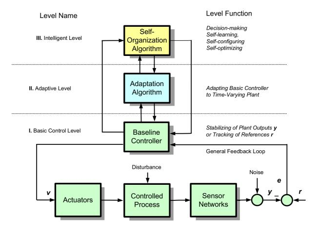
Fig. 2. General configuration of three levels hierarchical control system [8]
