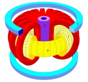
**Fig. 1.** Vertically elongated tokamak without an iron core: 1 is the vacuum vessel; 2 is the toroidal field coil; 3 is the poloidal field inner and outer coils; 4 is plasma and helical magnetic lines (© ITER Project Center, Russia)
