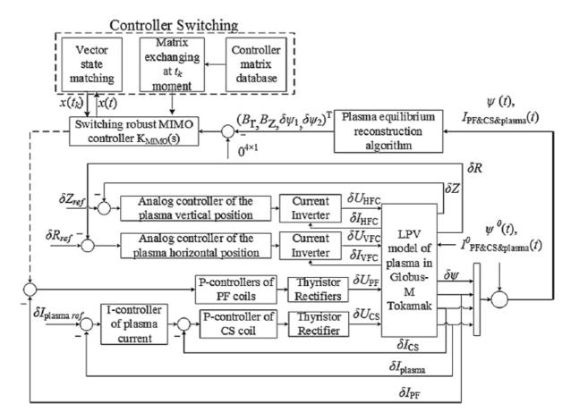
Fig. 6. Block diagram of multiloop and multivariable hierarchical plasma magnetic control system of the Globus-M2 tokamak [15]
