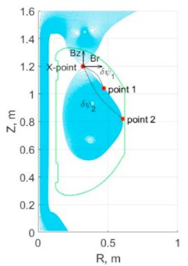
Fig. 7. The idea of the isoflux plasma shape control [15]
