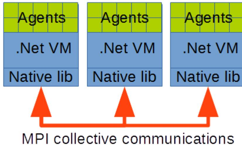
**Fig. 1.** The agents of the model are implemented using C# programming language and run in .Net virtual machine. The interaction between VM instances is implemented through the native library and MPI library.
