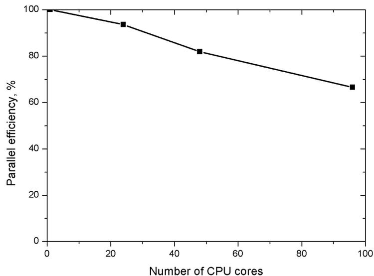
**Fig. 4.** The dependence of the parallel efficiency of the simulation on the number of MPI processes.
