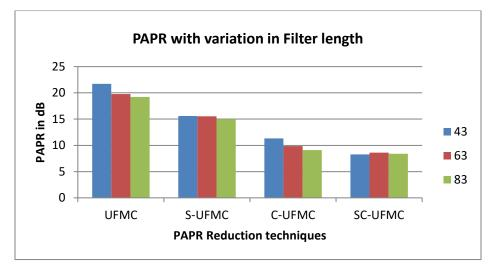
Fig. 5.4. Performance of various PAPR reduction techniques with different Filter lengths
