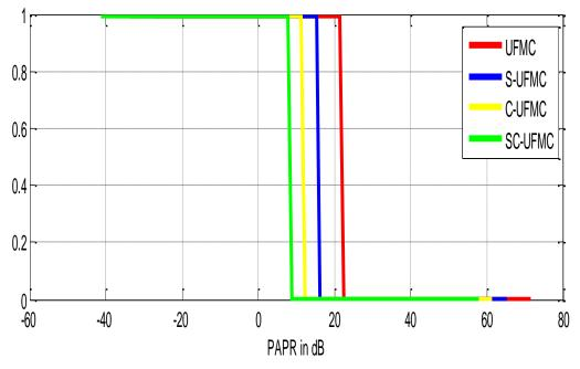
Fig. 5.1. PAPR reduction of different schemes
