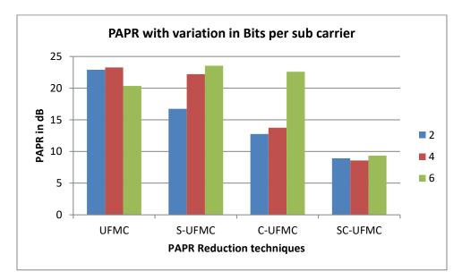
Fig. 5.3. Performance of various PAPR reduction techniques with different Bits per sub carrier
