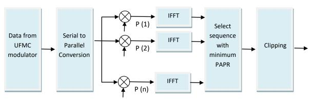
Fig. 4.1. Block Diagram of Hybrid (SC-UFMC) technique
