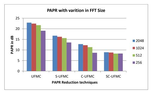
Fig. 5.2. Performance of various PAPR reduction techniques with different FFT Sizes
