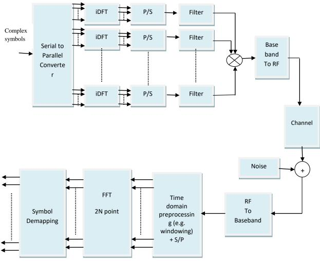
Fig. 2.1. UFMC Transceiver
