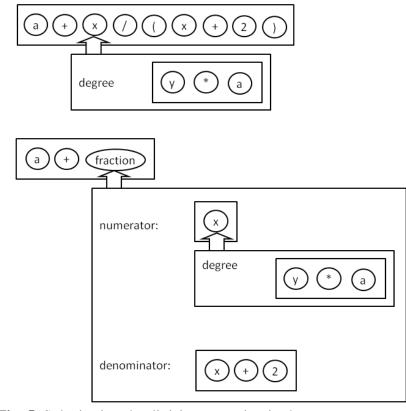
Fig. 5. Substitution the division operation in the computer memory
