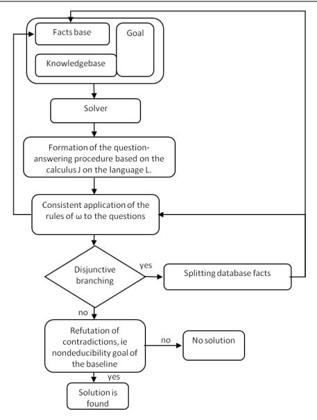
Fig. 2. Algorithm for finding the solution of the problem
